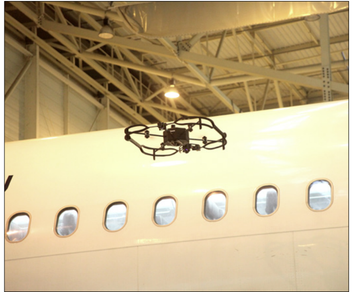
A Donecle drone performs an autonomous inspection of a commercial aircraft at the Air France hangars in Toulouse, France. Image via Wikimedia.
